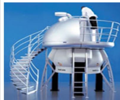
This is a machine used to do NMR spectroscopy. Most of these machines use magnets that are 500 megahertz to 900 megahertz. This magnet is 900 megahertz. Credit: Varian NMR Systems.
